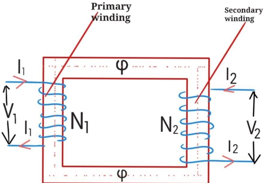
$$\frac{V_1}{V_2} = \frac{N_1}{N_2} = \frac{I_2}{I_1}$$
